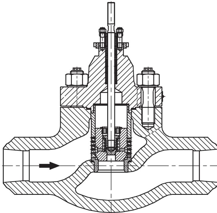
Fig. 1c. Valve Z1B - balanced plug with pilot.
