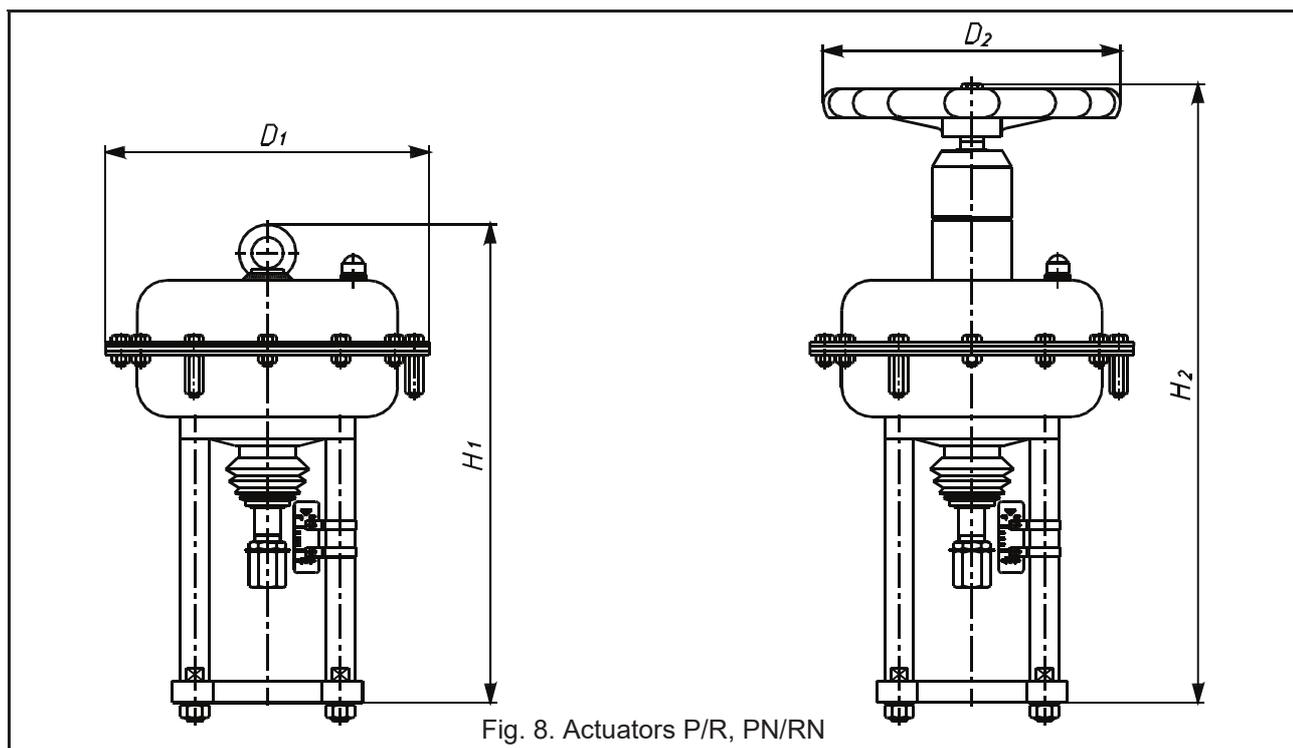
Fig. 8. Actuators P/R, PN/RN
